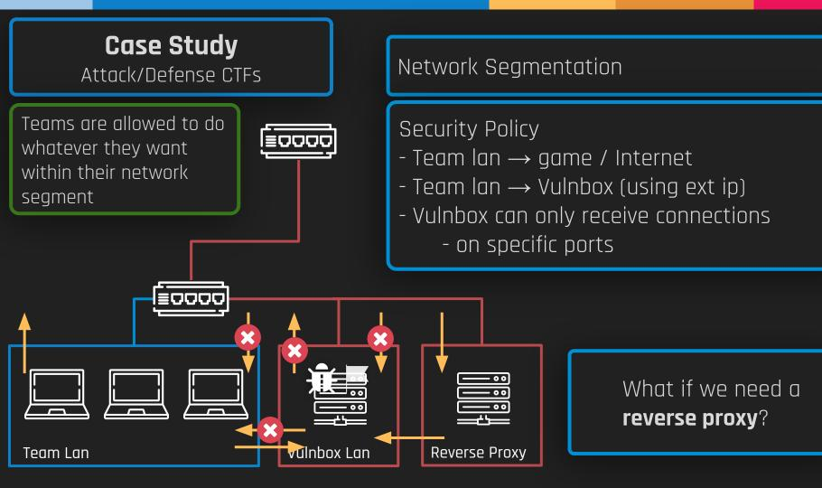
iptables -P INPUT DROP iptables -P FORWARD DROP iptables -A INPUT -m state --state ESTABLISHED,RELATED -j ACCEPT iptables -A FORWARD -m state --state ESTABLISHED,RELATED -j ACCEPT
